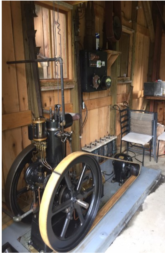
Fairbanks 4 HP hooked up to generator with glass jar batteries
